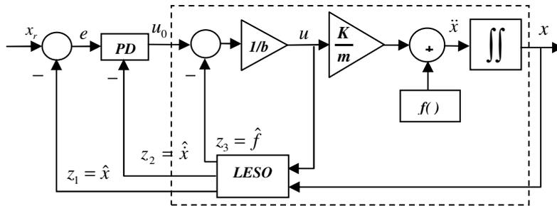
Fig. 2. Active Disturbance Rejection Control + PD position control
